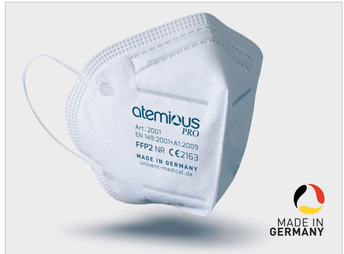
This close-up shows a finished Atemious Pro FFP2 medical respirator. Embossed areas show ultrasonic welds, which are used to bond multiple layers into the outer rim of the mask, contain the foldable nose-piece, attach the earloops, and form the curve that shapes the front of the mask. Photograph courtesy of Univent.
