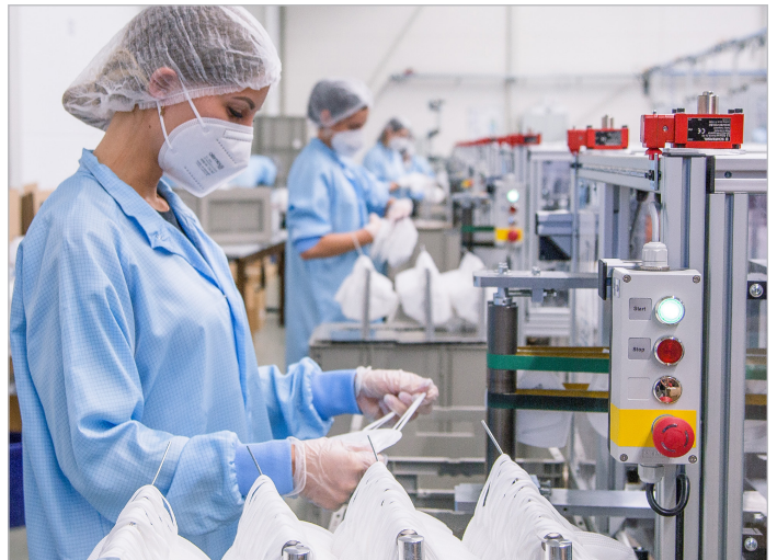
Completed Atemious Pro FFP2 respirators are removed from the production line, inspected and readied for packaging. Photograph courtesy of Univent.
