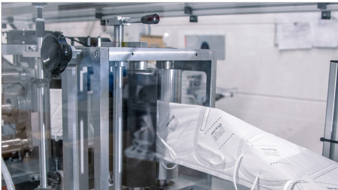
After ultrasonic welding equipment bonds multiple fabric layers together and attaches earloops, nearly completed respirators are folded and cut to the finished shape. Photograph courtesy of Univent.
