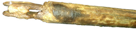
Figure 1-5. A Vibrating Fork Showing Severe Build Up and Bridging. Diagnostics Can Help Indicate This Issue Before Operation is Affected
