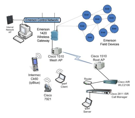
Network performance-analysis tools (an Iperf client and server) were connected to the test access points to provide a load on the Wi-Fi network. To provide voice over Internet protocol (VoIP) traffic, a Cisco 7921 IP phone and an Intermec CK60 mobile worker platform with a voice application were used.
