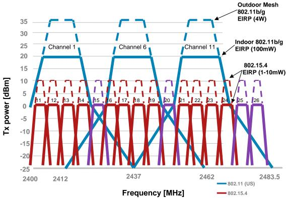
The diagram below shows areas of potential interference between transmissions using IEEE 802.11b/g (Wi-Fi) and IEEE 802.15.4 radios.
