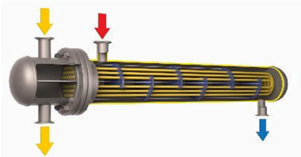
Figure 2. With a typical shell-and-tube heat exchanger, steam (red arrow) enters the shell and heats the process fluid in the tubes. Normally, it is designed to condense during these processes and leave the equipment (blue arrow) as condensate.
